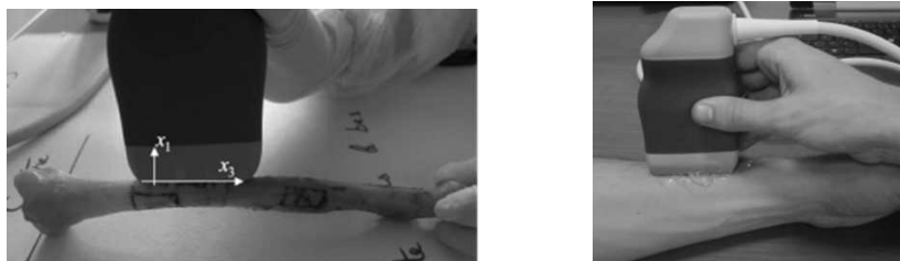
Figure 1: Ex vivo (left) and in vivo (right) measurement with the custom made multi-element probe
