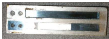
Figure 1: An accordion reed plate of the type used in this study
