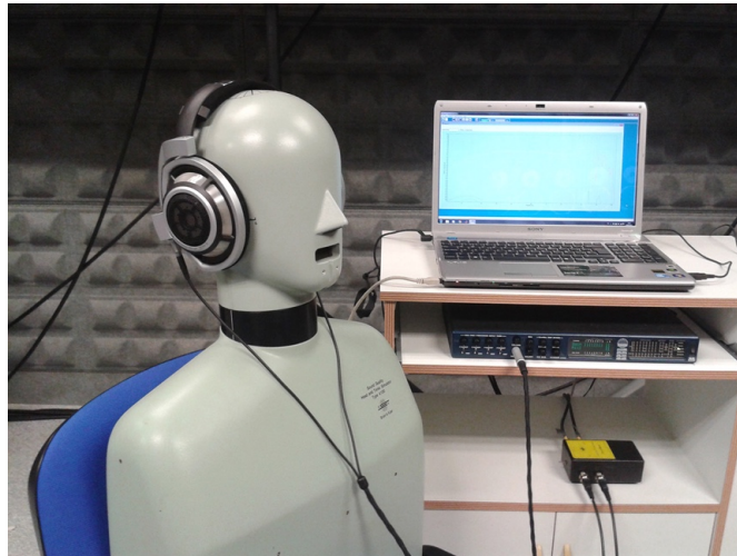
Figure 1: Set-up for measuring the headphones with the Head and Torso Simulator (HATS).
