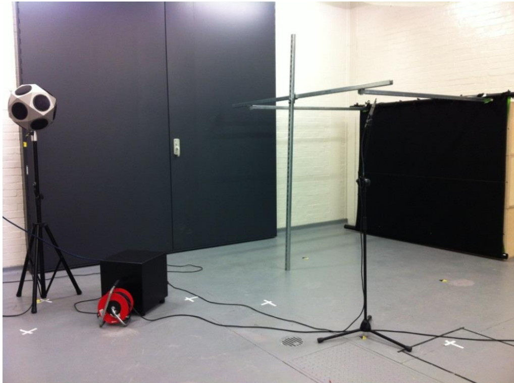
Figure 11: Variable absorption system
